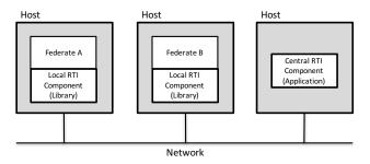
Figure 2: Physical deployment of an HLA federation
