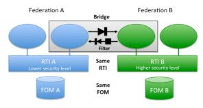
Figure 8: Segment federation into different security levels
